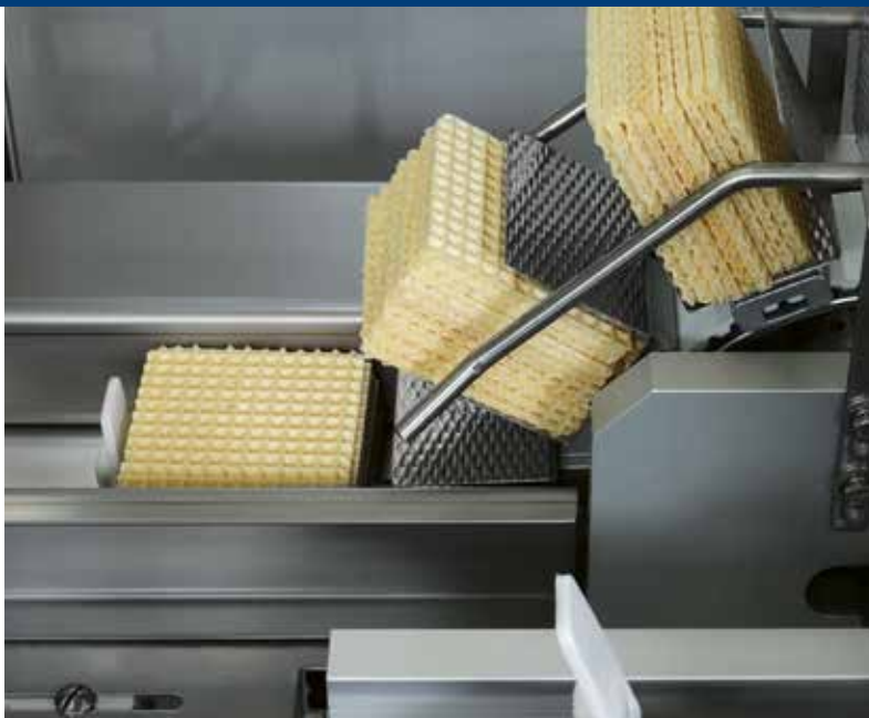
Overturning of the products to on edge position
