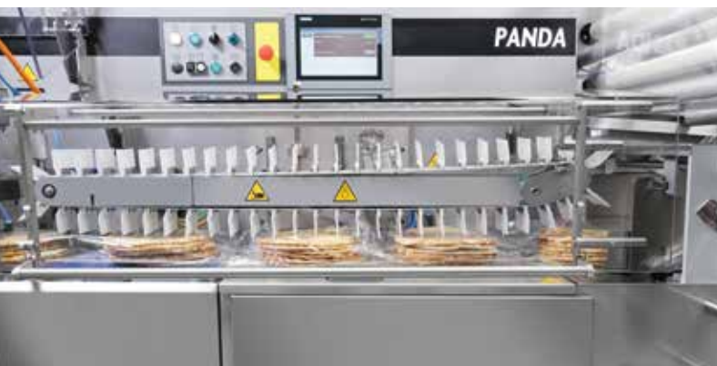
Overhead driven conveyor system
