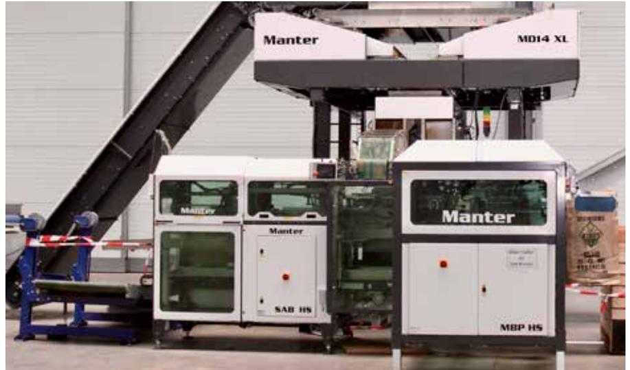
*Machines such as the MBP HS automatic bag placer in combination with the SAB HS bag sowing machine save the Luxembourg-based cooperative a lot on labour work.*
